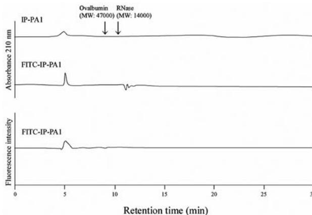
Figure 2. Elution profile of FITC-IP-PA1 gel filtration chromatography using HPLC. The column was eluted by 100 mM ammonium acetate at 25°C at a flow rate of 1 ml/min.
