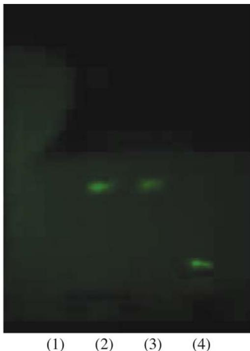
Figure 1. Thin layer chromatogram of FITC-IP-PA1. Samples were applied as 5  $\mu$ l spots, and developed in ethyl acetate. After development, the plates were dried and visualized using UV trans-illuminator (see Materials and Method). (1) IP-PA1, (2) FITC, (3) FITC and IP-PA1 mixture, (4) FITC-IP-PA1.
